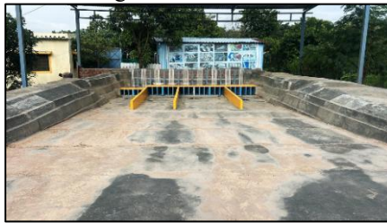
Fig. 3. Physical model with 3 divide walls
