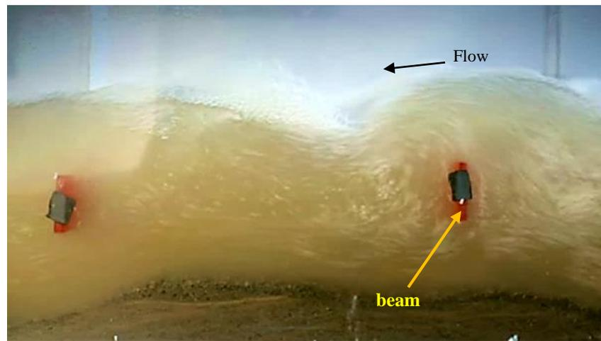
**Photograph 10.** Movement of sediment due to turbulence created due to Tees and Beam
