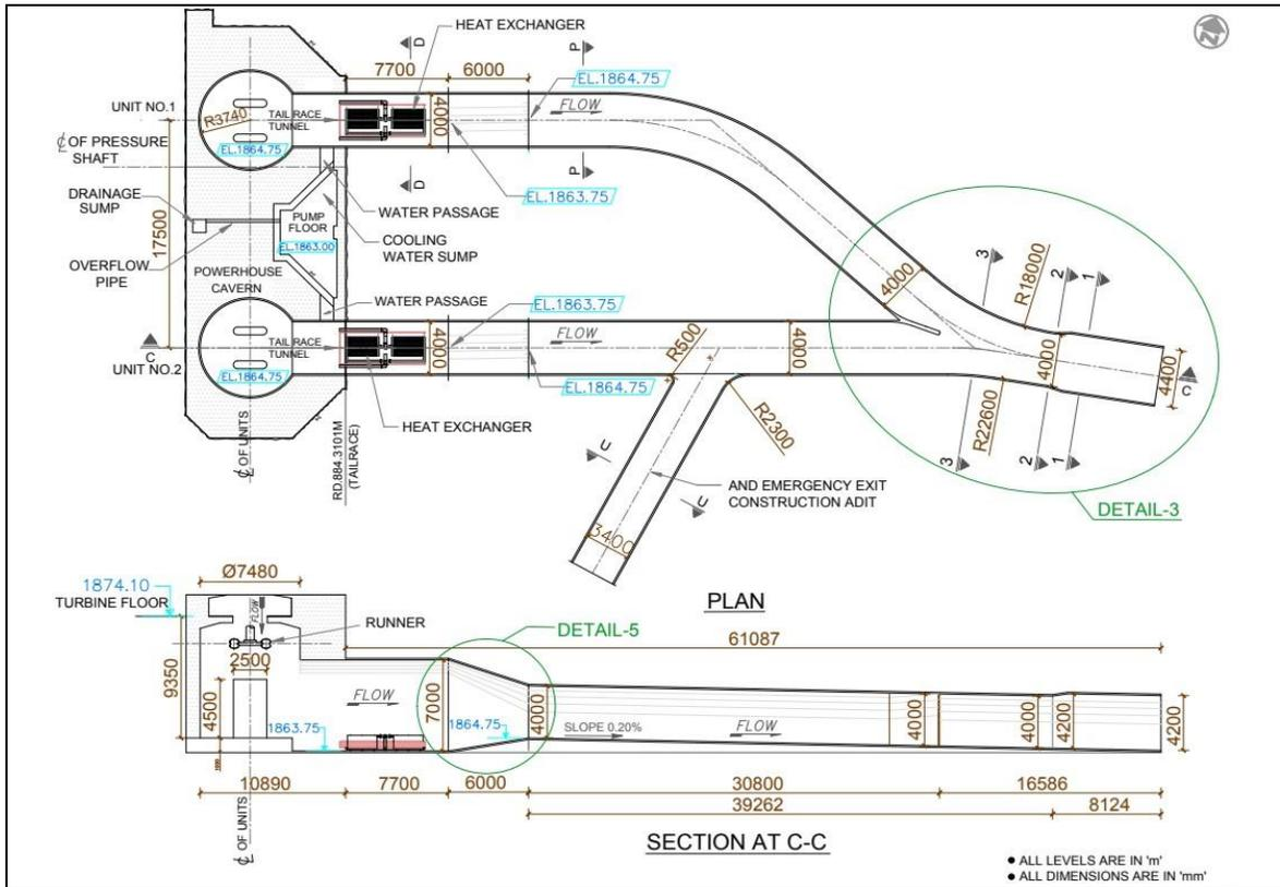
**Figure 1.** Layout plan and longitudinal section of Cooling water system arrangement in the tail race tunnel at the HPP
