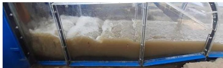
**Photograph 8.** Flow pattern observed after introducing of Tees and Beam
