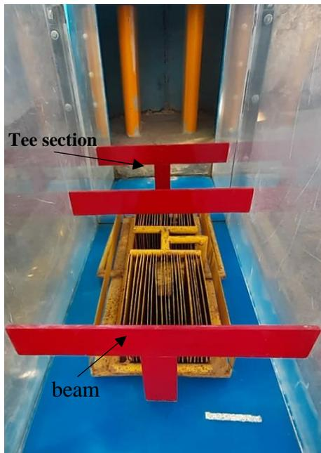
**Photograph 6.** Front view of model showing Tees, Beam and Heat exchanger unit
