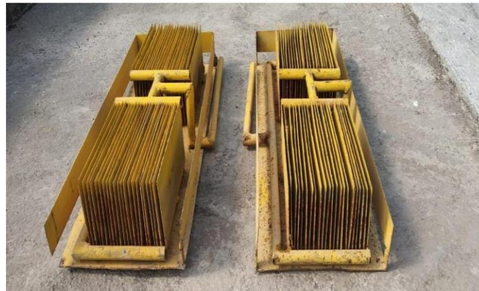
Photograph 4. Heat Exchanger units reproduced out of Mild Steel
