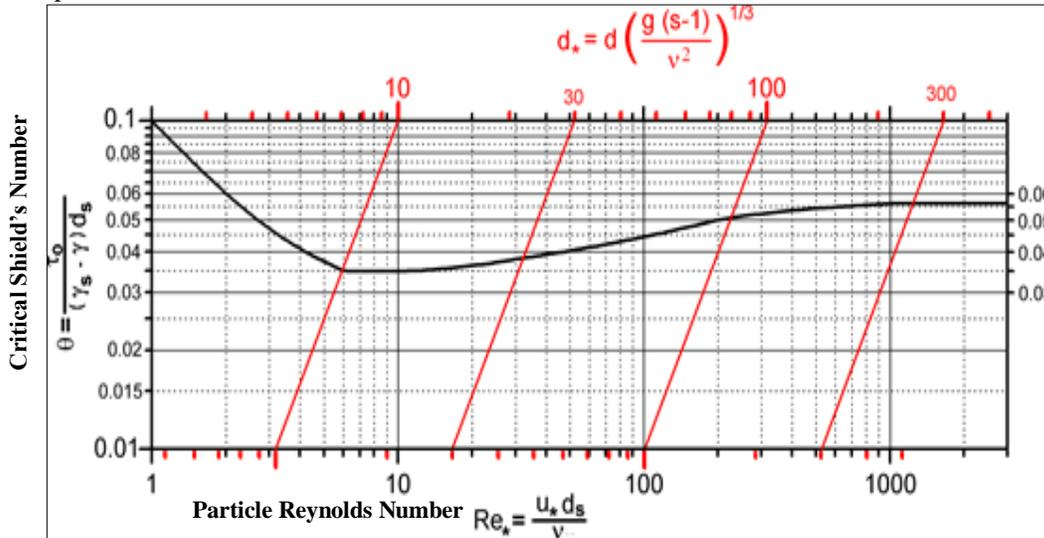
Figure 3. Shield's Diagram for sediment incident motion
