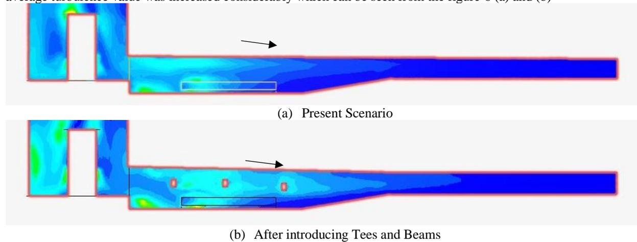
**Figure 6.** CFD studies for TRT showing increased turbulence after introduction of Tees & beam
