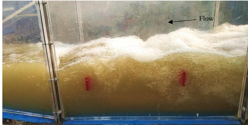
**Photograph 9.** Movement of sediment due to turbulence due to Tees and Beam
